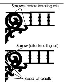
To complete a bracket installation to vinyl siding, apply a bead of caulk on both sides of the bracket where the bracket meets the siding. If you are not experienced applying caulk use masking tape to help create a neat appearance. Place the tape back from the edges approximately  $\frac{1}{4}$  in. Remove the tape before the caulk dries.
