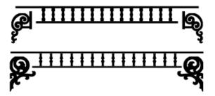
The first configuration is a single span with one rail section. (Left illustration) This configuration is used for spans up to 95" wide.
